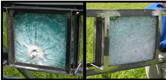
50 cal API round penetrates thick glass laminate
