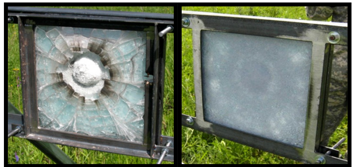
50 cal API round stopped by thin ALON ® laminate
